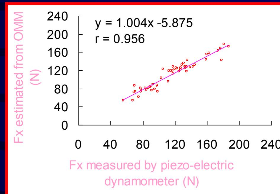
It can be seen that, notwithstanding the assumption that  $\delta_{other} \approx 0$ , the correlation is acceptably high ( $r$ -value is 0.956). It indicates that the machine tool can be made to act as its dynamometer from workpiece on-machine measurements performed on the same cutting machine!
