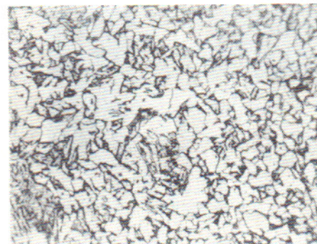
Fig. 4 Photomicrograph of the Cross Section of a Secondary Chip (x800) at High Positive V_t/V_w while Machining Low Carbon Steel
