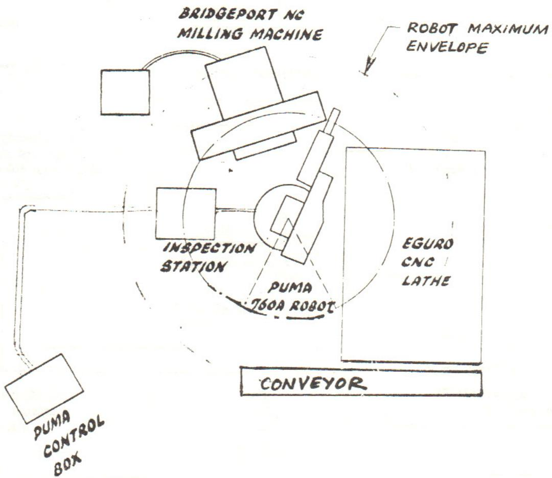
FIGURE 2 - LAYOUT OF FLEXIBLE MANUFACTURING CELL
